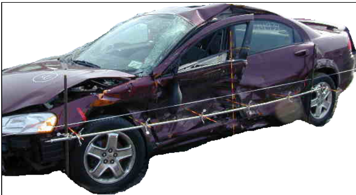
Figure 4.23: Deformation pattern of the struck vehicle, case#17
