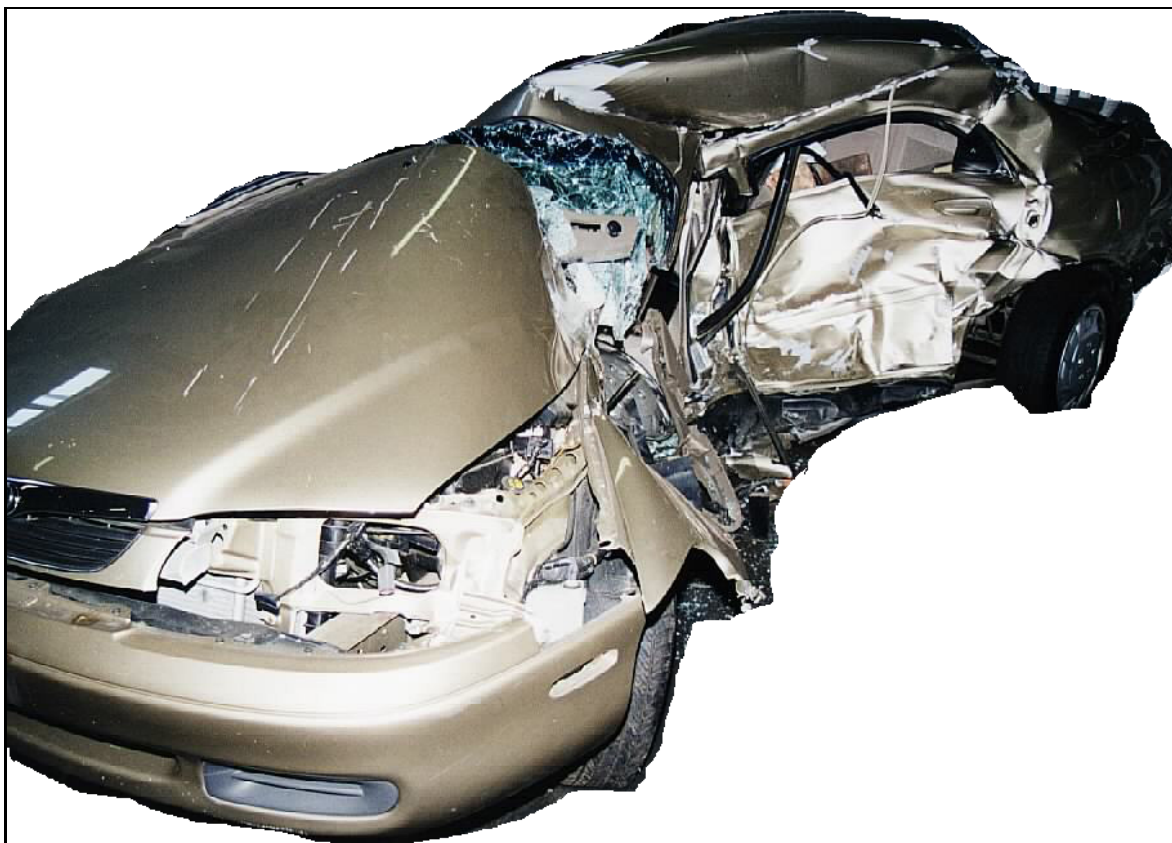
Figure 4.20: Deformation pattern of the struck vehicle, case#16
