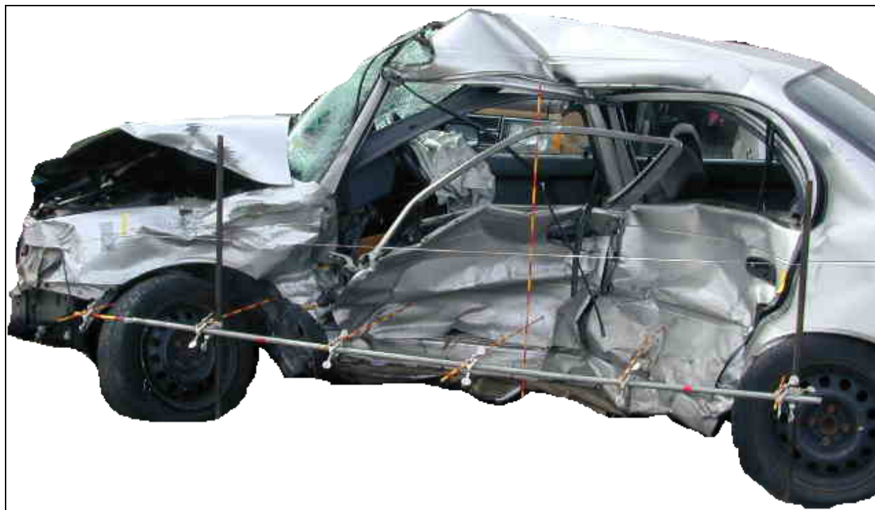
Figure 4.11: Deformation pattern of the struck vehicle, case#7
