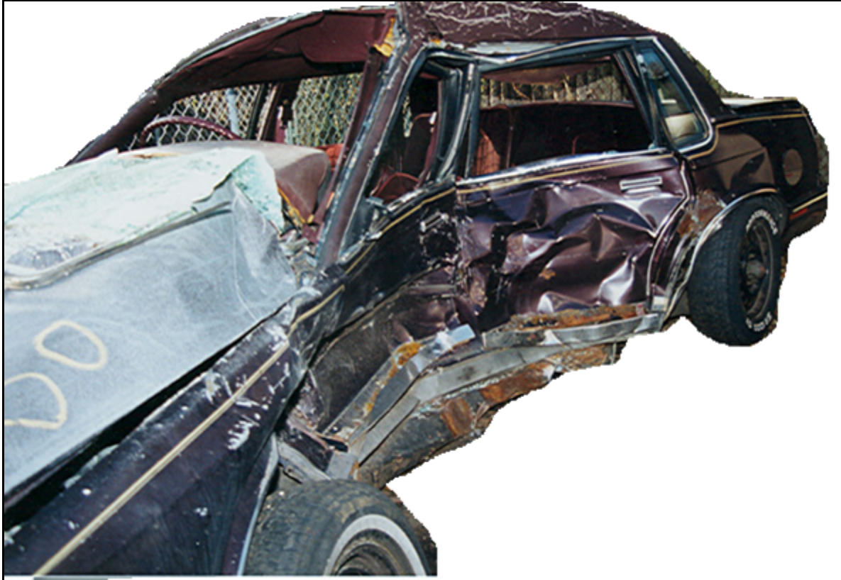
Figure 4.17: Deformation pattern of the struck vehicle, case#15
