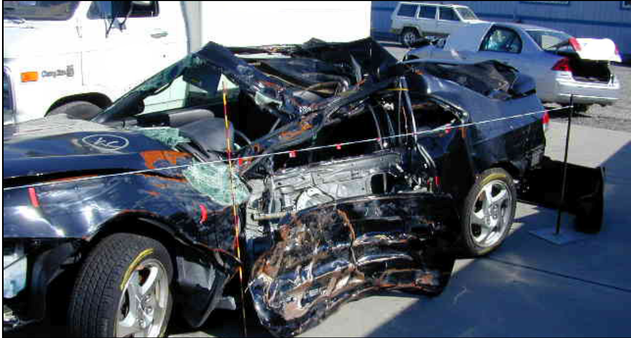
Figure 4.5: Deformation pattern of the case vehicle, case #5
