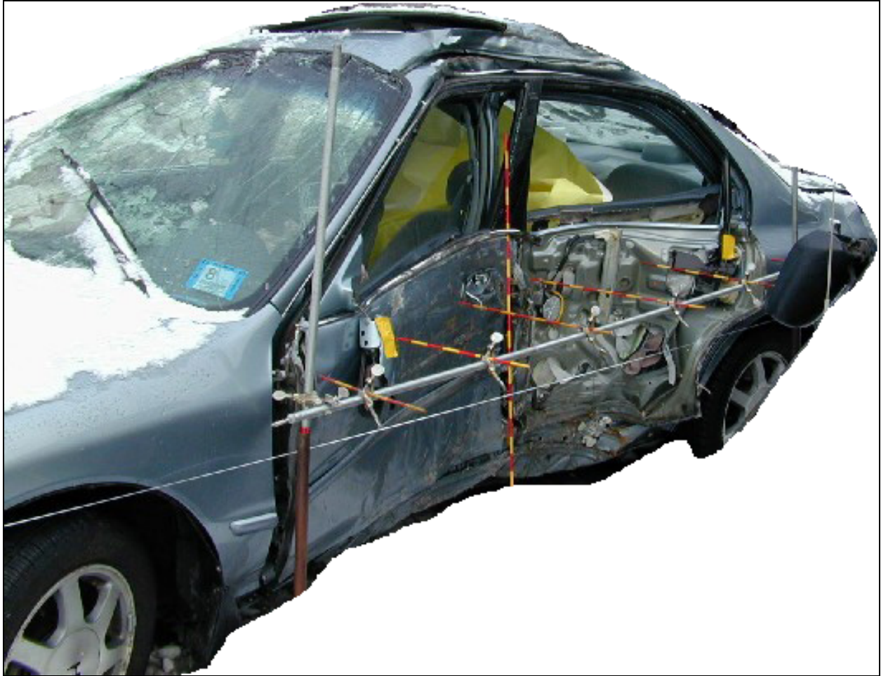
Figure 4.14: Deformation pattern of the struck vehicle, case#8
