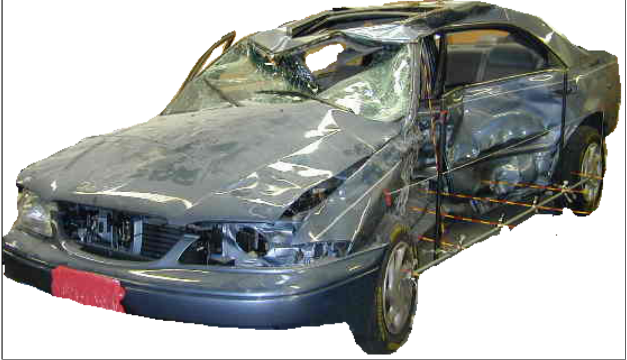
Figure 4.8: Deformation pattern of the struck vehicle, case#6
