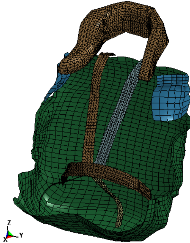
Figure 9.5: Seat, six-point harness system, shoulder support pads, and head support
